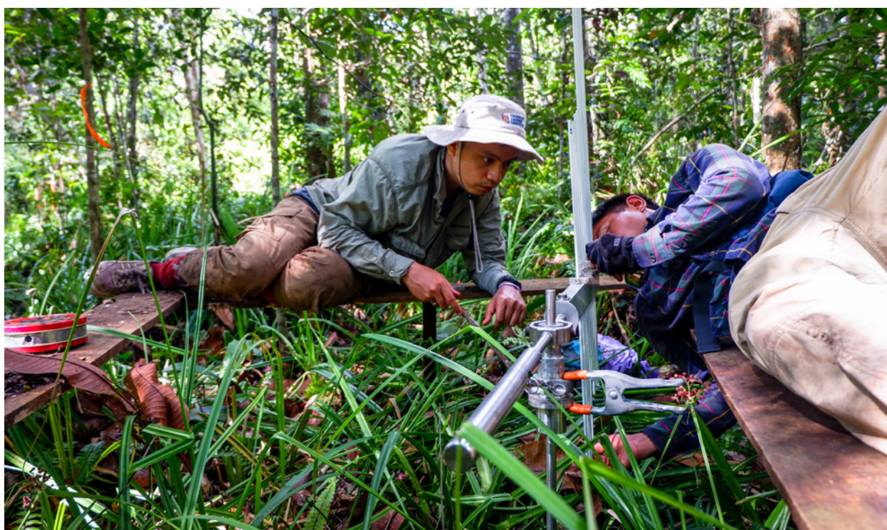
Researchers measure peat surface elevation change in Central Kalimantan, Indonesia.
